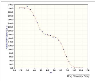
**Figure 3.** Plot of  $\mu_{eff}$  vs pH for quinine, indicating the presence of two different  $pK_a$  values.
