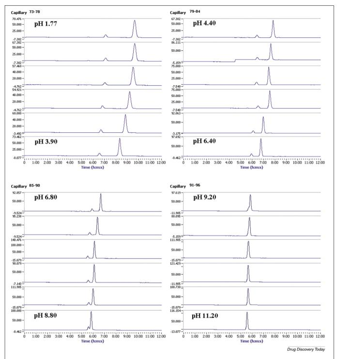
Figure 2. Simultaneously collected electropherograms at 24 different pH values for a sample of 100 ppm quinine (peak 1) with 0.1% DMSO (peak 2). A series of phosphate, formate and borate buffers of equal ionic strength (I=50 mM) were used to collect the CE data.
